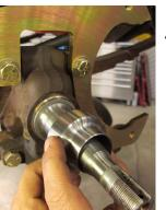
4. Install the supplied bearing adapter onto the spindle; if adapter doesn't fit snug (too loose should require spindle replacement), use green Loc-Tite sleeve retainer. Lightly hit with emory cloth if fit is too tight. (Fig 9)
