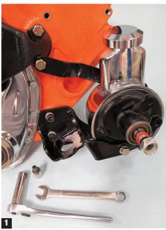
2. Unbolt stock bracket; replace with #PS808 using supplied cap screw Allens and lock washers. Install new motor mounts at this time if necessary. (Fig. 3)
