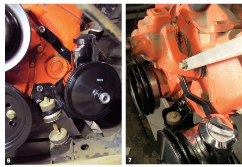
Verify the fit of your belts with the bracket positions; generally, a 15466 sized V-belt works best with a #CP38810 (PS pump), #CP38813 (dual-groove water pump), and #CP38811 crank pulley configuration. Tighten all bolts/ nuts and adjust the belt tension as normal. (Fig. 8)
