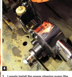
Loosely install the power steering pump (the open hooked end attaches to the lower rear stud on the pump, while the front bolts directly to pump as illustrated in Fig. 4).
