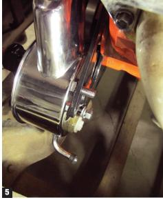
4. Loosely attach the adjusting arm bracket to the front of the pump and the engine. For "short" water pump applications, the dogleg points towards the pump; for "long" water pump applications, the dogleg in the bracket goes towards the engine. (Fig. 5)
