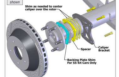
9. In some cases, the leaf spring plate might be in the way so you will need to install the lower rear bolt through the spacer, shim and bracket first before putting it on the axle housing. (Fig. 6)
