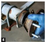
7. Slide the backing plate shim on to the axle and re-install the axles into the rear end housing. (Used on 1955-64 axles only) (Fig. 3 & 4)
