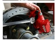
Note: Due to variations in the caliper castings, you may need to file down a small amount of metal on the bridge of the caliper if it rubs the outer edge of the rotor. See picture at right.
