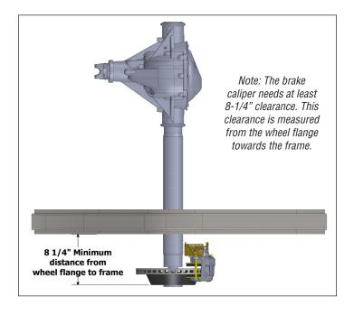
PLEASE NOTE: The installer needs to make sure that nothing can make contact with a brake hose, caliper, or other brake compo at any point through the entire range of steering and suspension movement. The installer also needs make sure none of the steering or braking components can become bound or jammed at any time through the range of suspension or steering movement.
