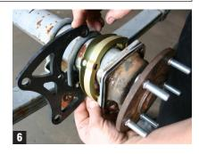
Tighten down the bracket to the housing end flange (Fig. 7). Install the right
