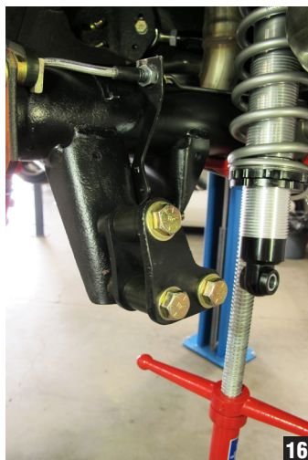
12. The four-piece lower mounting brackets are contoured to match the stock rear end—the dogleg will angle towards the front of the vehicle. Attach the lowest 1/2-inch bolt to the existing hole; using the bracket as a template, drill the upper 1/2-inch hole and attach supplied bolt. (Fig. 16)
