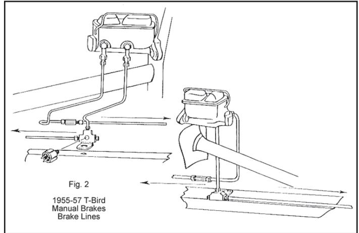
4. With the front brakes now complete, remove the rear steel brake line from the stop light switch block and install the supplied plug.
