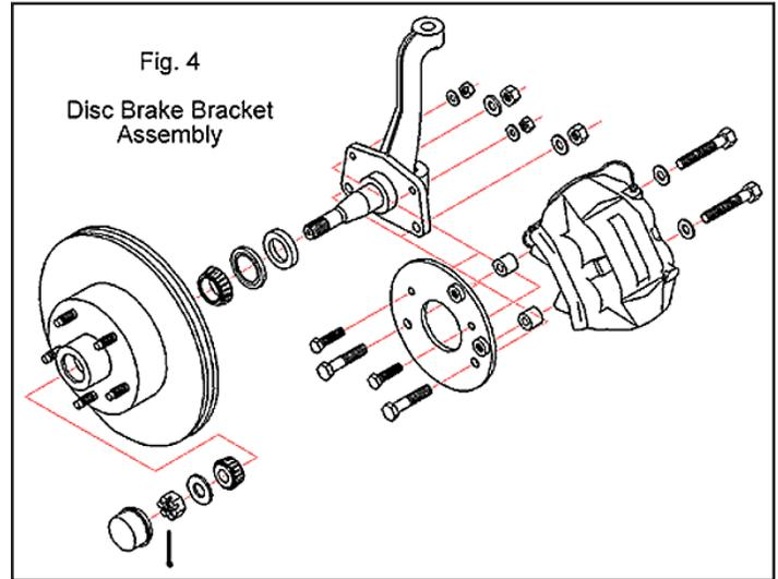
**WARNING!!** Stock drum brake wheels may not work with disc brake conversions. Drum brake wheels were not made with disc brakes in mind so there may be wheel to caliper clearance problems. Before installing this kit, make sure your wheels fit the brake assembly.
