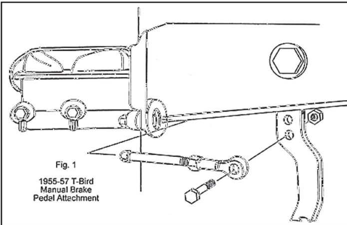
5. To attach the pedal to the new master, drill a 3/8" hole on the pedal 5/8" lower than the original mounting hole and install the supplied brake push rod. (See Fig. 1)
