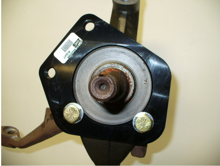
Spindle bracket mounting for Rear Steer applications
