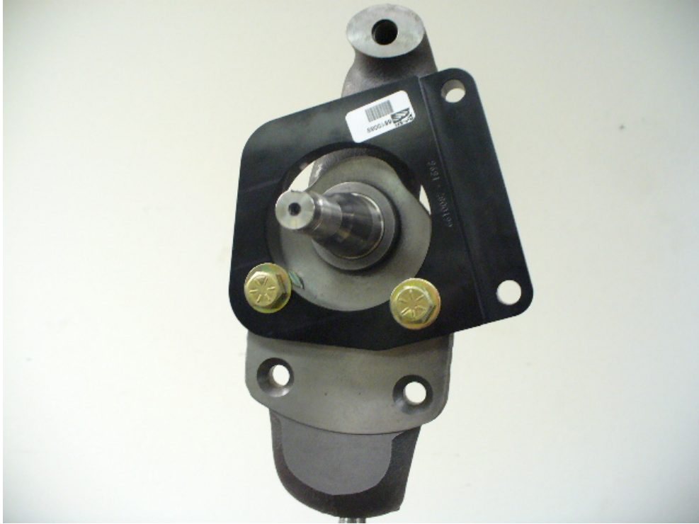
Bracket mounted on CPP drop spindle, spacers between bracket and spindle. Caliper position is behind spindle pin, this is the left (drivers) side.
