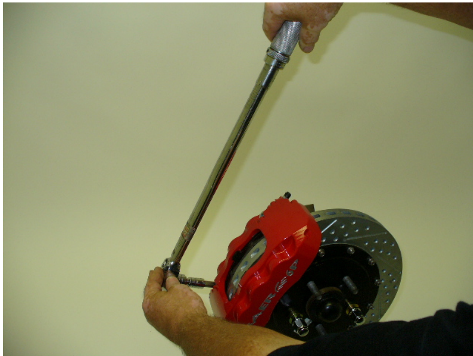
Torque caliper bolts to 85 ft-lbs.
