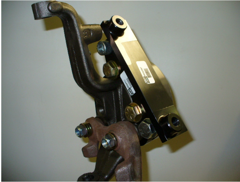
Radial mount bracket installed.
