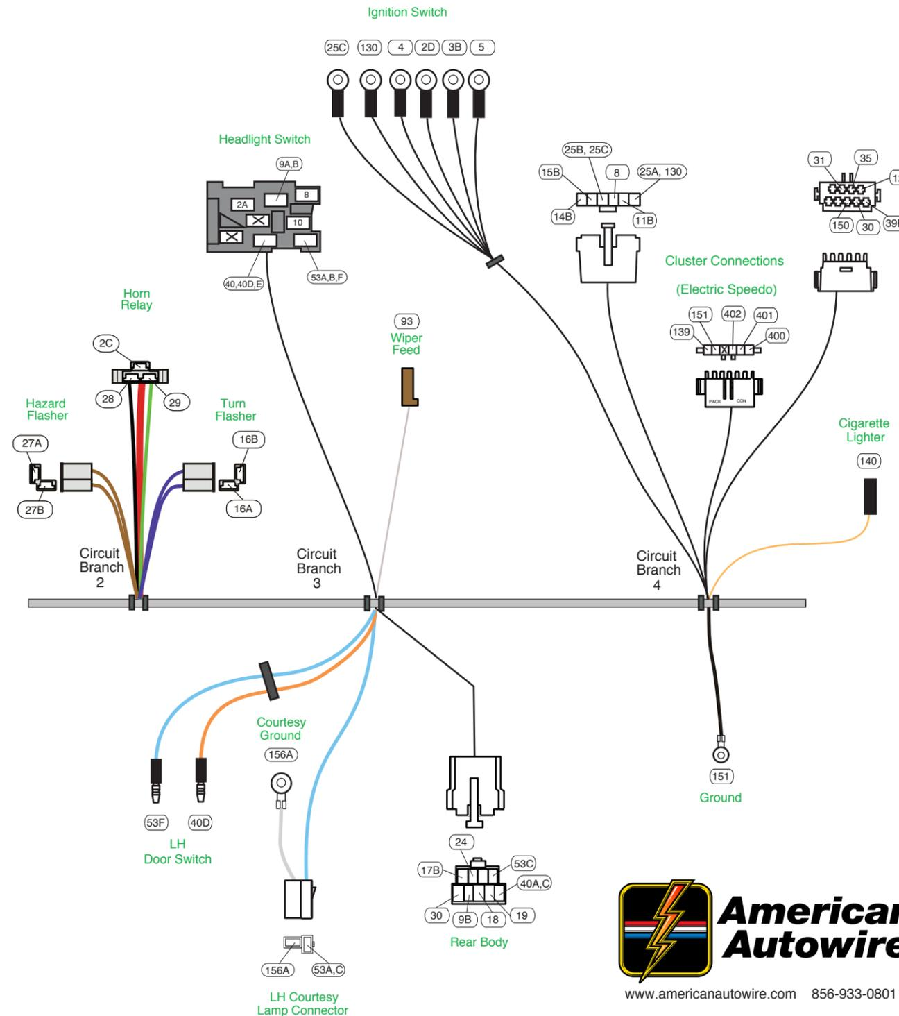
**NOTE:** The courtesy lamp extension from page 2, that plugs onto the connector at branch 3 on this page, uses a # 631 bulb (not included with this kit). They may be purchased at any auto parts store.
