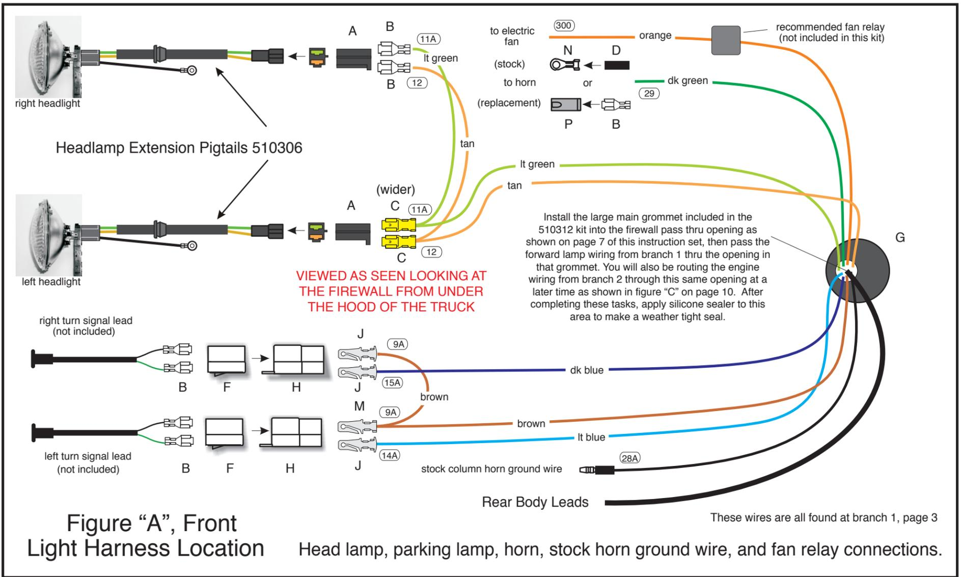
**NOTE:** The terminals and connectors listed on this page and denoted with **UPPER CASE LETTERS** to help you complete the various connections to your lamps, horns, switches, etc. can be found in your loose piece clamp, grommet, and parts kit, P/N 510312.
