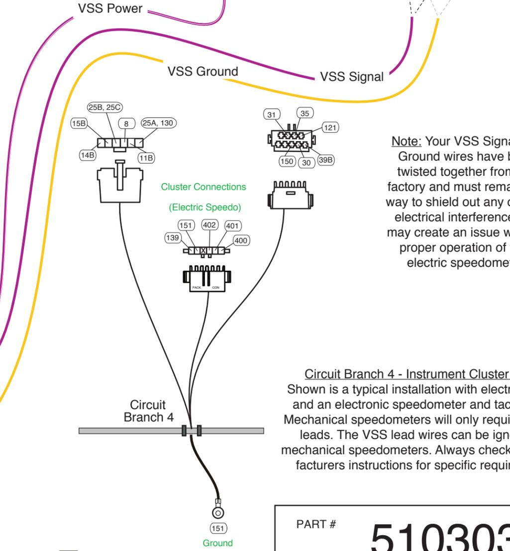
Circuit Branch 4 - Instrument Cluster Wiring
