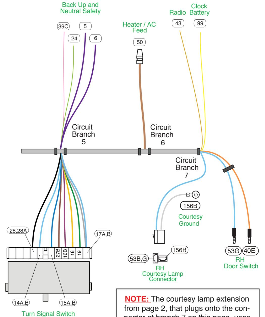
**NOTE:** The courtesy lamp extension from page 2, that plugs onto the connector at branch 7 on this page, uses a # 631 bulb (not included with this kit). They may be purchased at any auto parts store.
