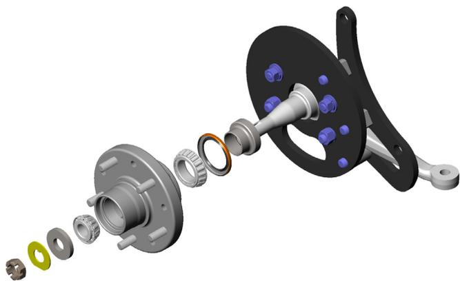
10. Install the bearing dust cap onto the hub. You may need to lightly tap the flange of the dust cap with a small hammer. Avoid hitting the domed part of the dust cap.
