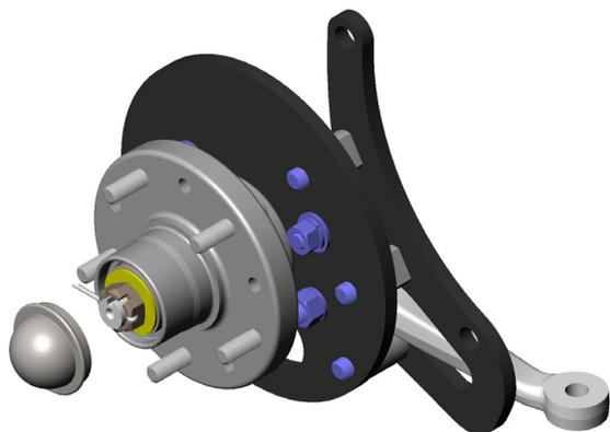
11. Install the rotor onto the hub assembly.
