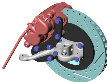
13. Check the rotors to make sure they can turn freely and the brakes are not dragging.
