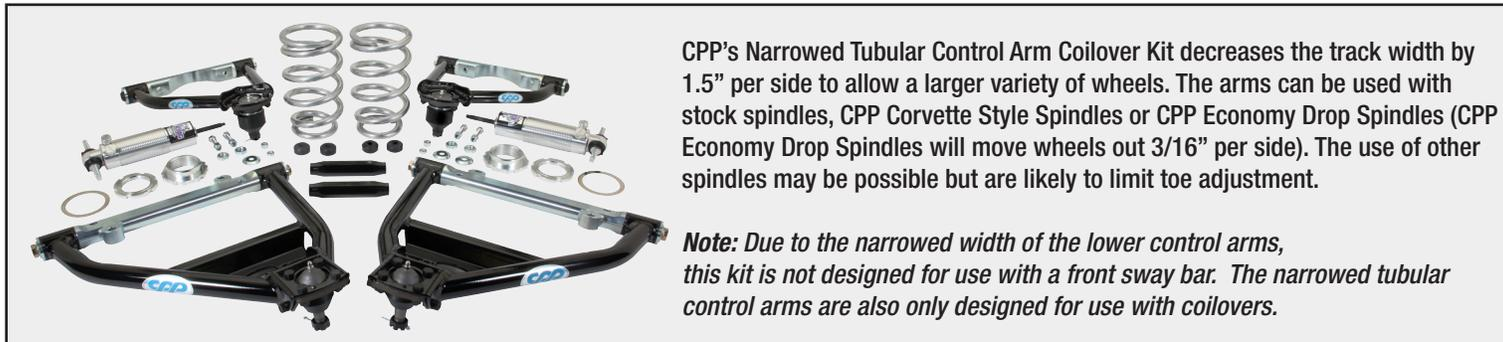
CPP's Narrowed Tubular Control Arm Coilover Kit decreases the track width by 1.5" per side to allow a larger variety of wheels. The arms can be used with stock spindles, CPP Corvette Style Spindles or CPP Economy Drop Spindles (CPP Economy Drop Spindles will move wheels out 3/16" per side). The use of other spindles may be possible but are likely to limit toe adjustment.
