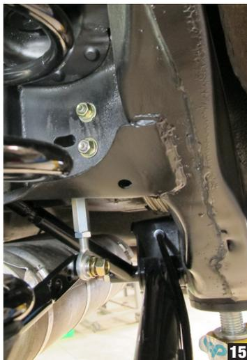
15. Once sway bar is set, secure axle clamps and bushing caps. (photo 18)
