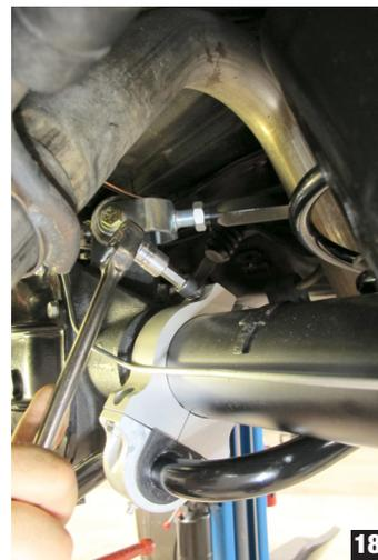
12. Attach upper bracket to frame using 3/8" hardware, including lock washers (photos 14 & 15).
