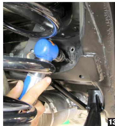
11. Providing there's sufficient room, using an angle drill and stubby bit, drill pilot holes for bracket from the front, mounting side; finish holes with 3/8" bit from the backside (photo 13).
