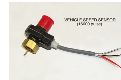
Typical 3 wire Autometer 5291 VSS connection
