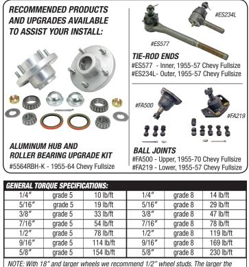
NOTE: With 18" and larger wheels we recommend 1/2" wheel studs. The larger the wheel diameter, the greater the force is on the wheel studs. Please inquire about replacement wheel stud kits available from CPP.
