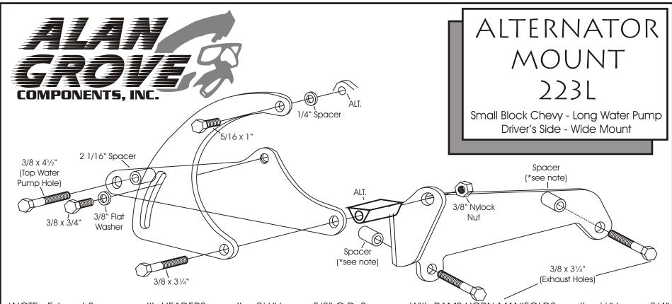
\*NOTE: Exhaust Spacers - with HEADERS - use the  $2\frac{1}{4}$ " long x 5/8" O.D. Spacers. With RAMS HORN MANIFOLDS use the  $\frac{1}{4}$ " long x 3/4" O.D. Spacer at rear hole of bracket and a 1 1/16" long x 3/4" O.D. Spacer at front hole of bracket. With the later DROP-TYPE MANIFOLDS use the 1 1/16" long x 3/4" O.D. Spacers at both bracket holes. As with any mount system, assemble all of the brackets to engine BEFORE tightening the bolts.
