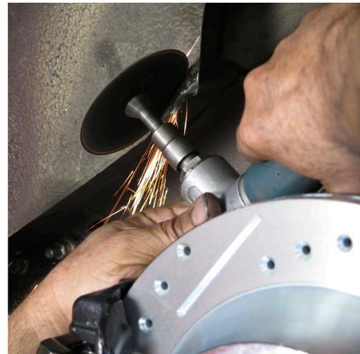
For 1968-69 Camaro / Firebird and 1968-74 Nova / X-body cars, it may be necessary to clear the drivers side frame as shown to avoid the caliper making contact.
