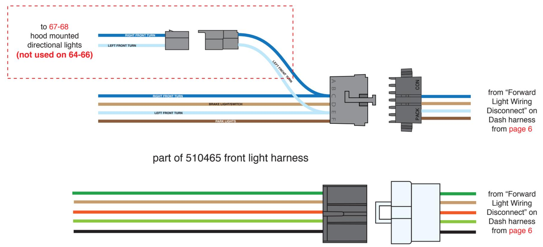
these wires are to be routed thru forward lamp wiring firewall pass thru opening (see page 19)
