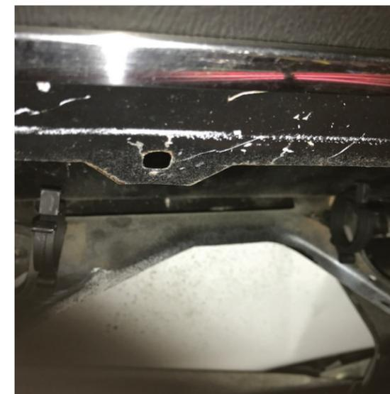
5. Install the two harness routing clips "N" into the original holes near the top of the two vertical dash supports as shown above.
