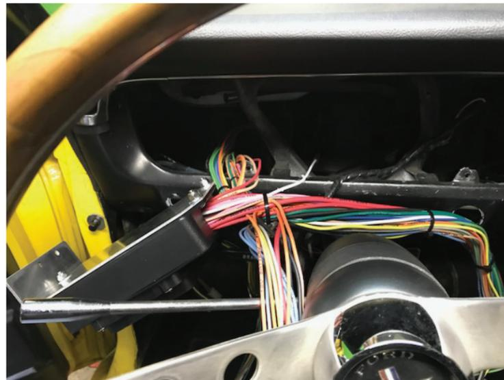
3. With the cluster assembly and all the original wiring removed, lay the assembled "bracket, fusebox and harness assembly" from step 1 across your steering column as shown above.
