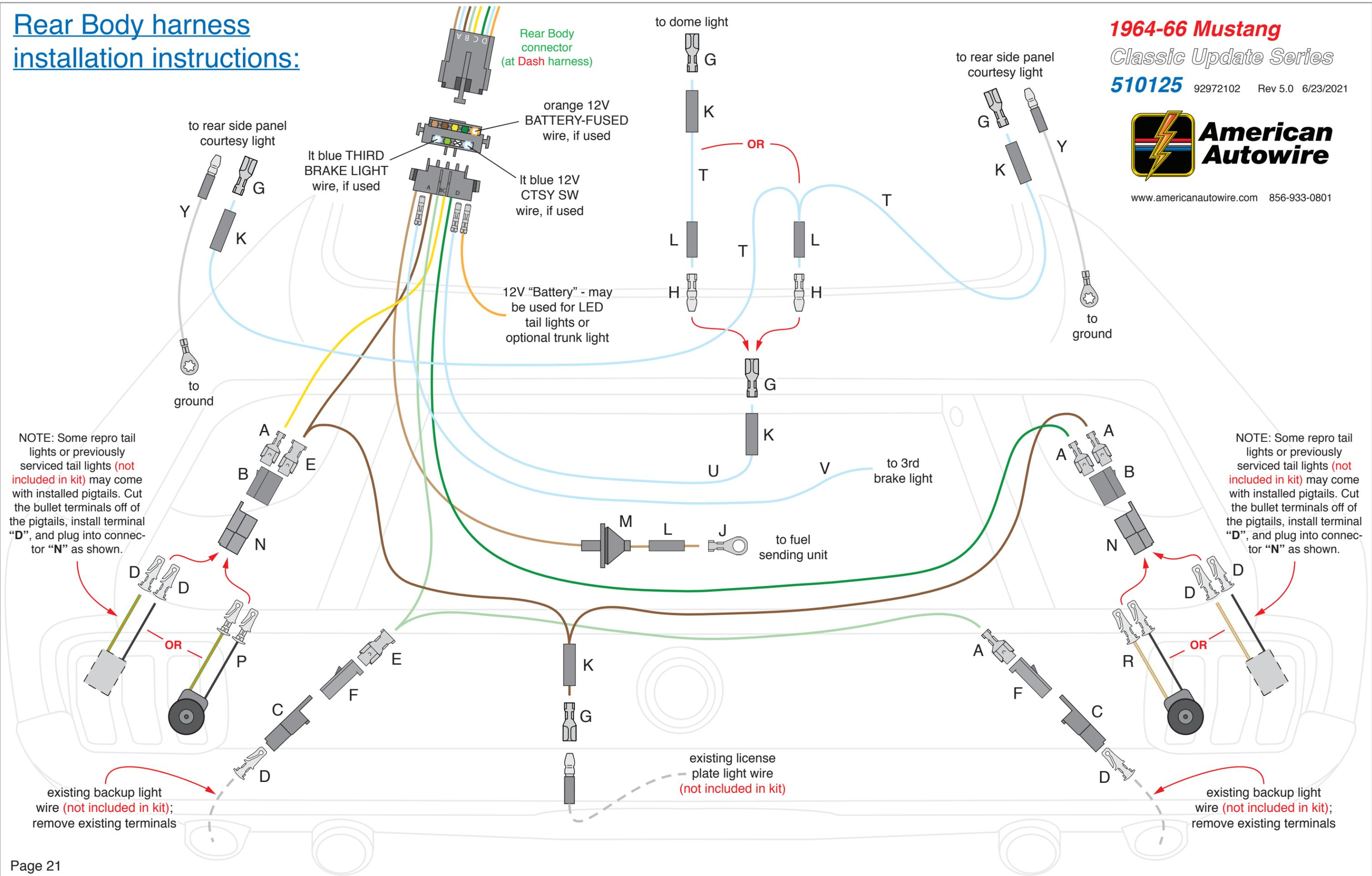
NOTE: Some repro tail lights or previously serviced tail lights (not included in kit) may come with installed pigtails. Cut the bullet terminals off of the pigtails, install terminal "D", and plug into connector "N" as shown.
