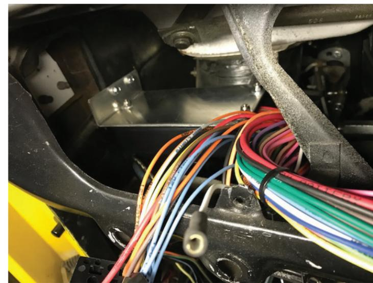
4. Tuck the "bracket, fusebox and harness assembly" down inside the dash opening, and using screws and washers "F and G" found in the 92972060 dash loose piece kit, attach the assembly to the LH door hinge pillar area. Carefully route the harness to avoid any sharp edges on the LH vertical dash support so that you do not cut or chaff any wires.
