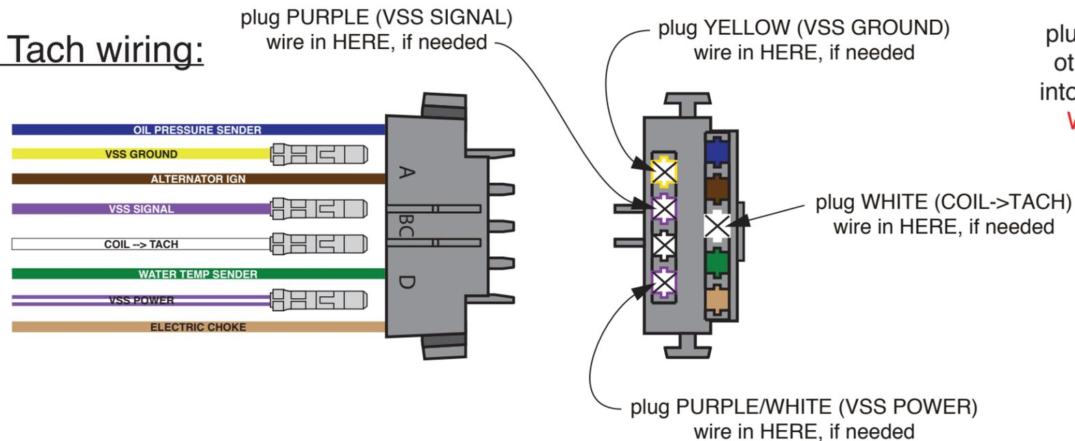
plug this connector (along with the other Engine harness connector) into the Dash harness (see "Engine Wiring Disconnect" on page 6)
