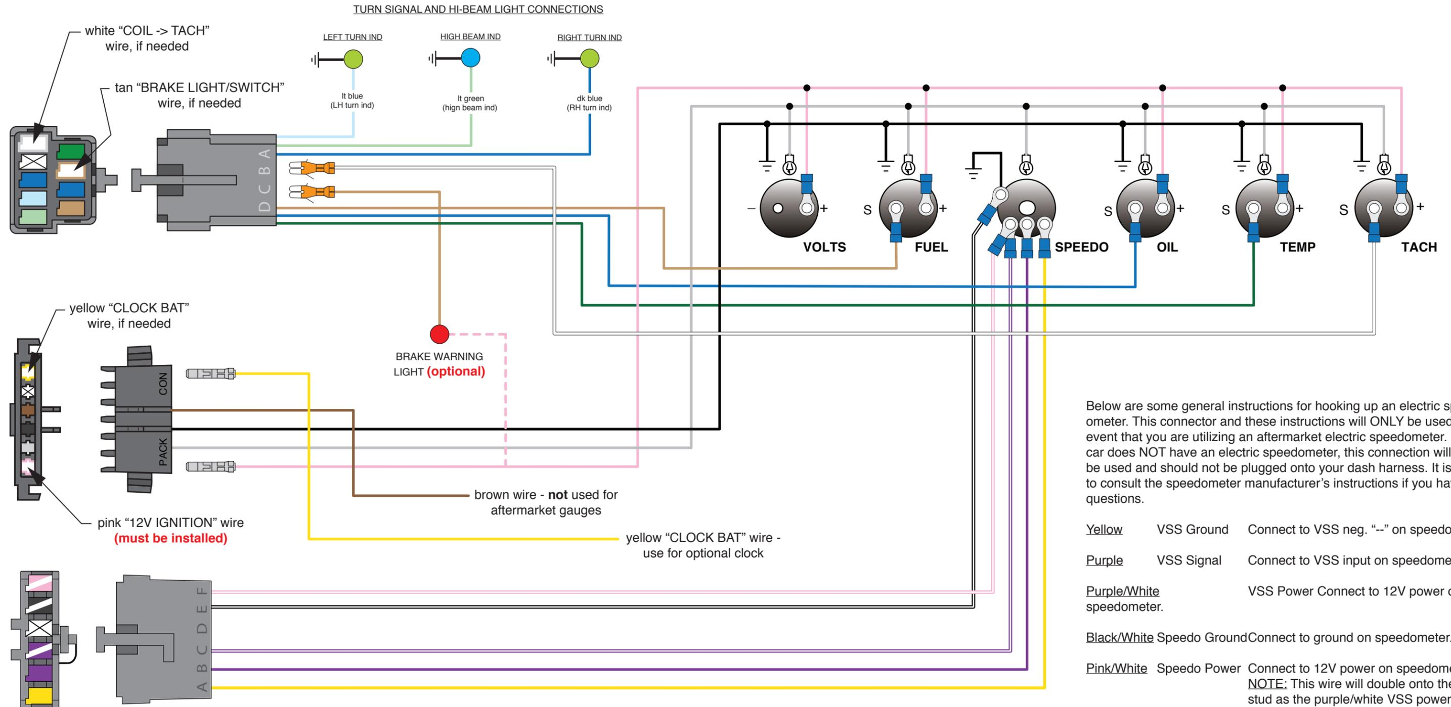
Below are some general instructions for hooking up an electric speedometer. This connector and these instructions will ONLY be used in the event that you are utilizing an aftermarket electric speedometer. If your car does NOT have an electric speedometer, this connection will NOT be used and should not be plugged onto your dash harness. It is best to consult the speedometer manufacturer's instructions if you have any questions.
