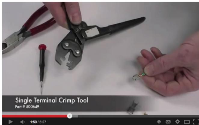
The terminals that we supply in our kits, utilize what is known as an F crimp. The F crimp, in a cross section, will look like the illustration below, when done correctly.
