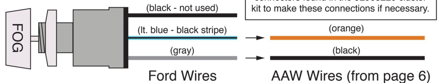
**NOTE:** The factory Ford fog lamp switch utilized 3 wires: blue with a black stripe, gray, and black. For this application, the AAW orange wire will be connected to the original Ford blue with black stripe wire, and the AAW black wire will be connected to the original Ford gray wire. The original Ford black wire will not be used in this application and should be capped off.
