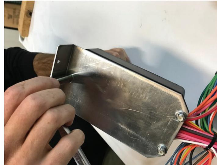
1. Assemble the mounting bracket to the fuse-loaded fusebox and harness assembly using screws, washers and nuts "H, J and K" found in the 92972060 dash loose piece kit.
