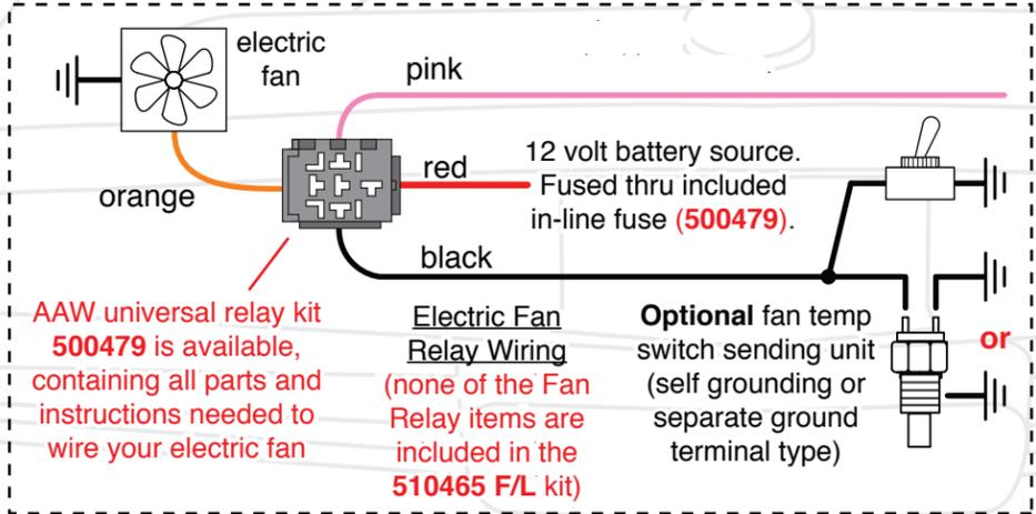
fused 12V ignition source for fan relay
