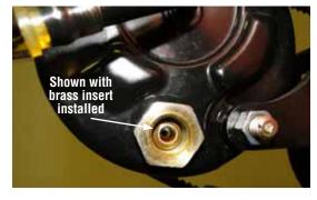
brass inserts installed, please discard the three supplied inserts. If you do need to install the brass inserts, use a small punch to tap the inserts in place.
