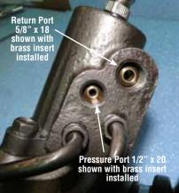
Be sure to use a line wrench to tightening down all fittings. Install the hoses into the rack. Tighten them down snug. **Do not over tighten**.
