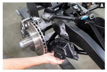
**WARNING:** Do Not remove the cross shaft pivot bolts on either the upper or lower tubular control arms; they are installed with Loctite. Removing the cross shaft bolts will void the warranty. (Photo B)
