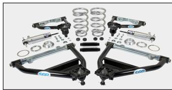
CPP's Narrowed Tubular Control Arm Coilover Kit decreases the track width by 1.5" per side to allow a larger variety of wheels. The arms can be used with stock spindles, CPP Corvette Style Spindles or CPP Economy Drop Spindles (CPP Economy Drop Spindles will move wheels out 3/16" per side). The use of other spindles may be possible but are likely to limit toe adjustment.
