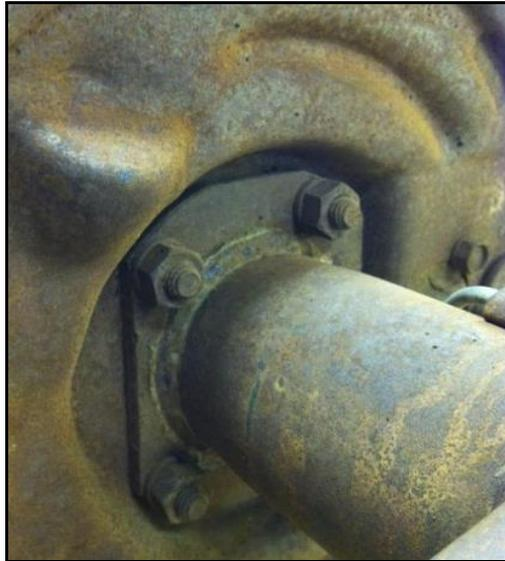
**Figure 3:** Photo shown of OE fasteners and OE backing plate
