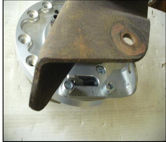
**Figure 5:** Park brake assem (inboard view)
