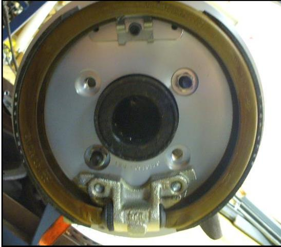
**Figure 4:** Park brake assem (outboard view)
