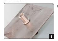
1. The Universal EZ-Return Rivet Fitting is essentially a rivet nut insert disguised as a bung. By tightening the provided Grade 8 fastener, once installed the body of the bung begins to collapse, securing the bung in place and providing a leak-free installation.
