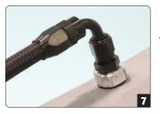
7. Here's the bung with the AN fitting and return line installed.
