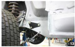
13. The new steering box has a special triangular mounting plate that is installed on the wheel well side of the subframe with the mounting bolts going through into the engine bay. Make sure this plate is installed here and not on the engine bay side. (Photo 13)
