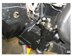
28. Once you confirm your upper measurement, it is now time to mark and drill the roll-pin hole. If you can accomplish this while in the car, you can simply drill the hole. If you have limited space, simply remove the inner shaft again and drill it out with a drill press. (Photo 28)
