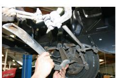
11. From the wheel well position, remove the stock mounting bolts to the steering box. Make sure to hold the gear box when removing the last bolt, so you don't drop it out, as the inner steering shaft inside the car could cause damage to the dash. Once loose, carefully lower the steering box out of the engine bay down from the bottom of the car. (Photo 11)
