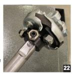
26. Slide the #6466FPK seal and mounting ring onto the steering column tube, prior to bolting the column into the car as shown. (Photo 26)
