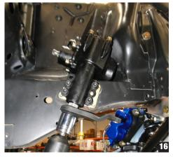
Install the retaining nut and washer, and torque down to properly seat the lock washer. (Photo 16)
