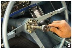
5. Before you remove the steering column out of the car take a measurement of how much the inner
