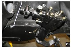
23. Install the rag joint onto the steering box. Remove the Allen head bolt from the rag joint and slide it onto the shaf. When the opening is visible though the hole in the rag joint, put the Allen bolt back through and tighten it up. Make sure it is tight enough to remove any slop. (Photo 23)
