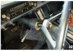
32. With the turn signal switch, spacers, and spring re-installed, you can now put the steering wheel back in place. Confirm the steering box and wheels are straight and centered, and mount the steering wheel back in center. (Photo 32)
