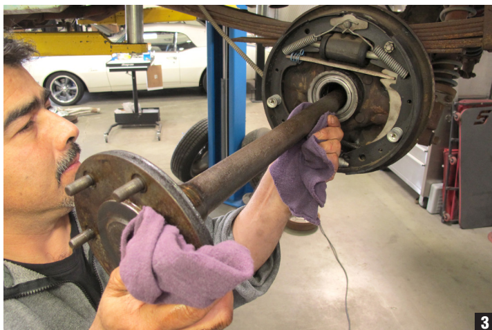
3. Carefully slide axles out; inspect for excess bearing surface and input spline wear. (Fig. 3)
