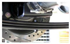
10. When installing the axle on the narrow leaf springs, line up the hole in the bottom of the spring pad with the dowel pin on top of the leaf.
