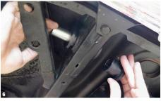
In the rear of the car, install the supplied D-Spec bushings and sleeves in the chassis before fitting the hanger brackets.
