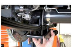
11. Next, install the U-bolts which secure the axle to the leaf spring using the tie plate.
