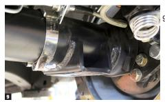
Once the pinion angle is set correctly and the axle is centered, weld on the supplied narrowed leaf spring pads.
