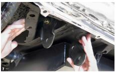
With the bushings and sleeves installed into the chassis, you can go ahead and loosely bolt on the hangar brackets.
