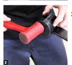
The bushings can be installed using a rubber mallet. Just make sure to line them up square and then tap 'em in.
