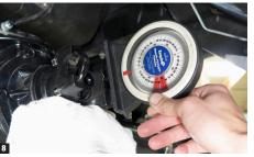
8. Then you'll need to check the angle of your engine and transmission and, with the vehicle sitting at ride-height, set the pinion angle.
