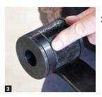
Here's a look at the bushing spacer when installed. It offsets the springs a half-inch inboard for more tire clearance. (You might notice we are using the D-Spec bushings in the front here instead of the supplied rubber ones. That's because we'll be installing traction bars which come with the upgraded bushings for the front spring eye.)
