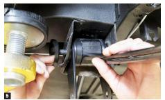
Next, hang the front of the leaf spring using the supplied hardware. (Again, you'll notice the D-Spec bushings and added brackets since we'll also be installing traction bars.)
