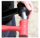
The last step for preparing the narrow leaf springs is installing the supplied sleeves. Like the bushings, the sleeves can be installed easily using a rubber mallet.
