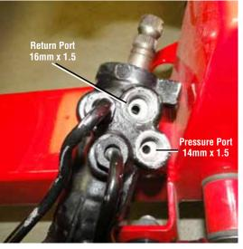
Be sure to use a line wrench to tightening down all fittings. Install the AN o-ring fitting adapters into the rack. Tighten them down snug. Do not over tighten. Be cautious as over time, many reconditioned rack fitting ports get worn and become weak, so its very easy
