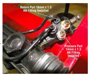
return port on the rack is the top one closest to the splined shaft. The pressure port is the one below it.
