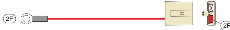
“EE” GM “SI” Alternator Exciter Wiring
