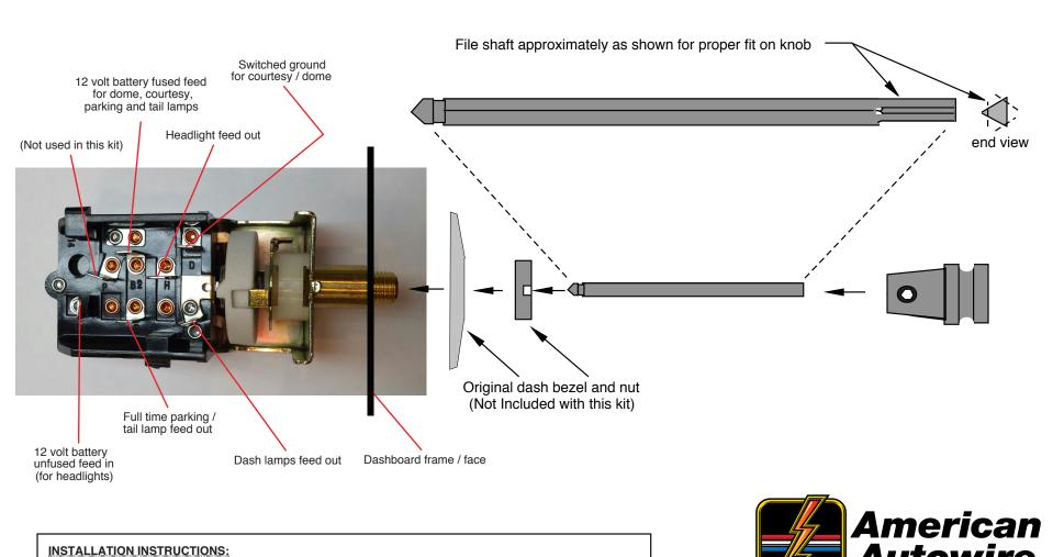
1. Install the new switch into your dash using the original bezel and nut. It will be necessary to cut the shaft for a nice custom installation. Please take note of the flat area cut onto the threaded brass mounting shaft of the switch, and the square edge cut into switch mounting area on the face of the dash. These two features are to help the switch index properly in the face of the dash.
