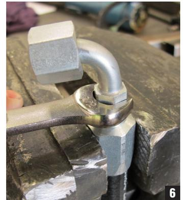
5. Once position is marked, place the hex collar in a vice and tighten down the fitting completely. (Fig 6)
