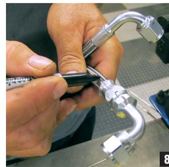
7. Before completing your fitting by fully tightening, mock up in the vehicle and position the fitting angle—mark with a Sharpie to help keep positioned. (Fig 8)
