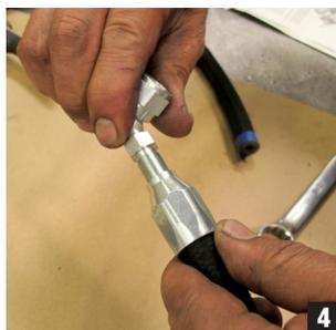
4. Before completing your fitting by fully tightening, mock up in the ve-
