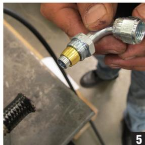
5. The male end of the compression fitting has a brass sleeve that slides over the male nipple—the taper should point away from the fitting. Inside the sleeve are graduated “steps”; the Teflon liner needs to be inserted firmly into the sleeve as it’s pressed on. (Fig 5-6)
