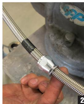
2. Slip female collar fitting onto the stainless line before cutting (threads pointed toward end to be cut), as it may want to fray freshly cut wire braid if done afterward. (Fig 2)
