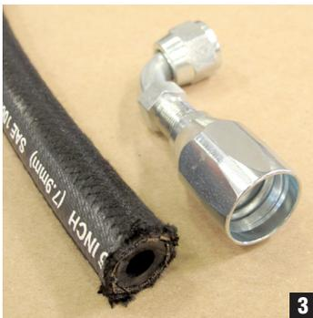
2. Beneath the cloth braid is a steel-meshed layer; you will need to use a cutoff wheel (or fine-toothed hacksaw) to cut the hose. Carefully trim any excess fray that may result. (Fig 2-3)
