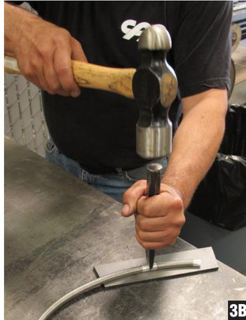
3. There are a few different methods in which to cut the braided stainless: preferably is by using a high-speed, thin-bladed cutoff wheel (Fig 3A); however, an extremely sharp chisel and heavy hammer also work well (Fig 3B), but care needs to be taken to “not” pinch the inner Teflon tube (a similar-sized punch can be used to reshape the Teflon after it’s been cut).
