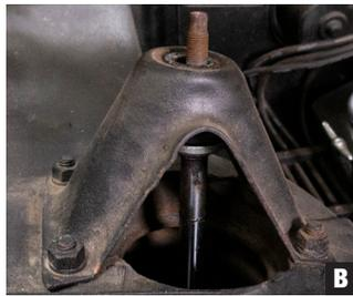
2. Then remove the shocks from the vehicle by removing the upper and lower shock mounts and the shock tower brackets (Photo B).
