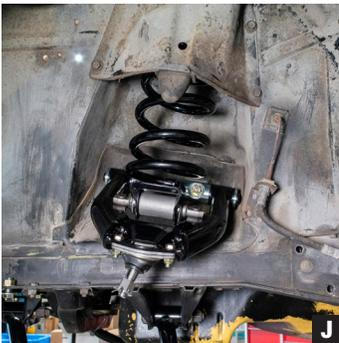
11. Ensure the spring is properly oriented in reference to the locating tab on the spring perch, then slowly release the tension on the spring.
