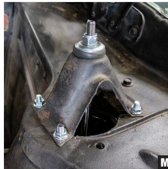
14. Put one of the supplied washers on the top of the shock followed by a bushing. Then re-install the shock tower, add another bushing and washer to the top of the shock, and finally secure with a nut.
