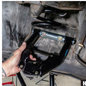
9. Install the new control arm using the supplied hardware. (Photo H)
