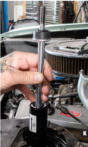
12. Install the new shock into the shock tower.
