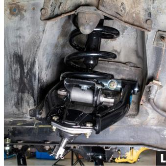
13. Fasten the shock to the spring perch using the supplied hardware.
