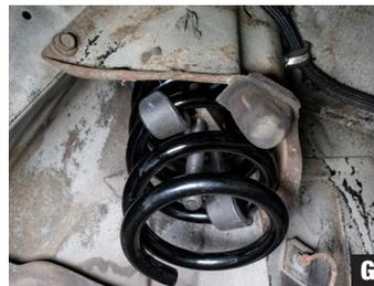
7. We suggest replacing the spring retainer plates (part number 6267CRP). Simply lift the plate into place and then a small turn will lock it in. (Photo F)
