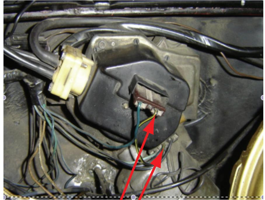
The photo above depicts the typical stock 1970-73 Camaro “with depressed park” wiper motor and washer pump connections. Where you see the black wire with the yellow strip in the photo, that would be equivalent to the AAW white “wiper feed” power wire.
