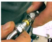
7. Before completing your fitting by fully tightening, mock up in the vehicle and position the fitting angle—mark with a Sharpie to help keep positioned. (Fig 8)
