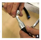
position the fitting angle—mark with a Sharpie to help keep positioned. (Fig 5)
