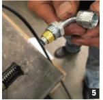
5. The male end of the compression fitting has a brass sleeve that slides over the male nipple—the taper should point away from the fitting. Inside the sleeve are graduated "steps"; the Teflon liner needs to be inserted firmly into the sleeve as it's pressed on. (Fig 5-6)
