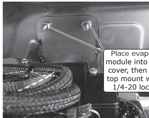
Place evaporator module into firewall cover, then secure top mount with (2) 1/4-20 locknuts
