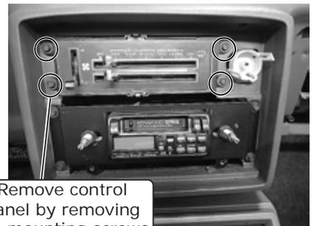
Remove control panel by removing (4) mounting screws
