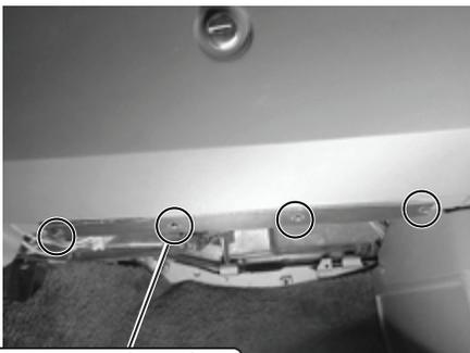
Remove glove box door by removing (4) screws
