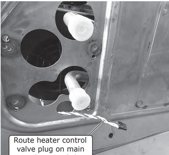
Route heater control valve plug on main wiring harness (white, yellow and purple) through firewall cover
