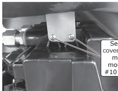
Secure firewall cover to evaporator module lower mount using (2) #10 x 5/8" screws
