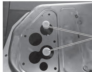
Place evaporator module into firewall cover and center heater hardlines
