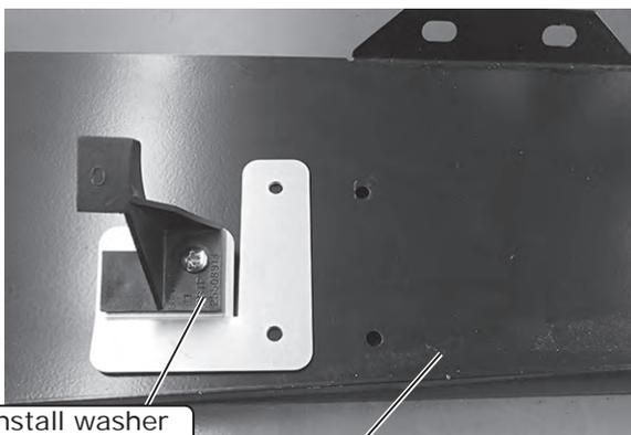
Install washer nozzle assembly onto water deflector
