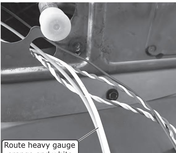
Route heavy gauge orange and white wires through firewall cover
