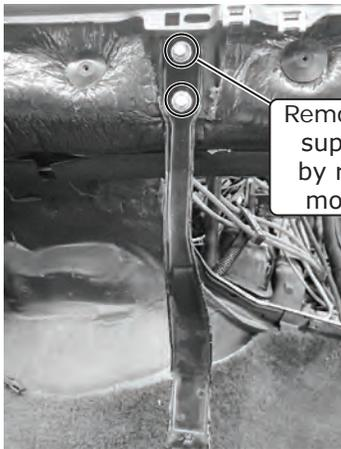
Remove OEM dash support bracket by removing (2) mounting bolts
