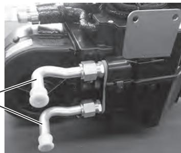
Loosely install (2) heater hardlines with properly lubricated #10 O-rings
