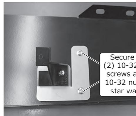
Secure using (2) 10-32 x 1/2" screws and (2) 10-32 nuts with star washers
