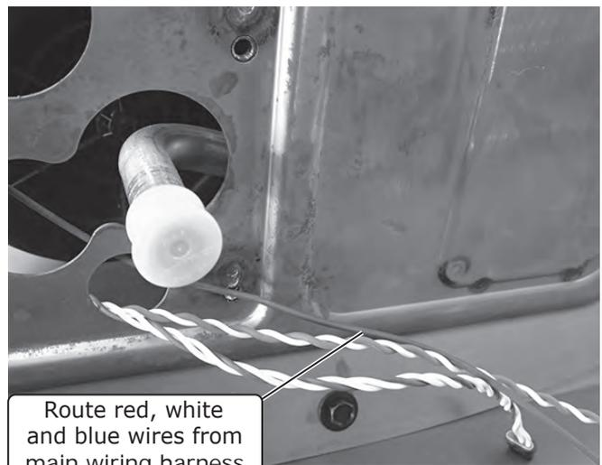
Route red, white and blue wires from main wiring harness through firewall cover
