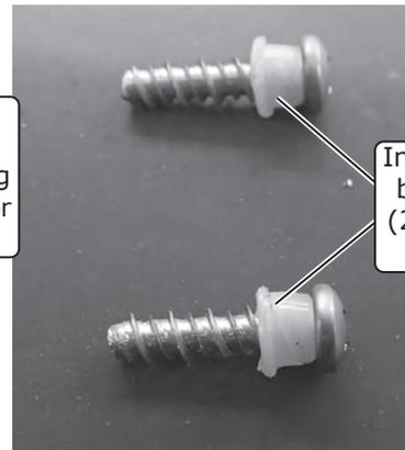
Install (2) nylon bushings onto (2) 8-18 x 5/8" screws
