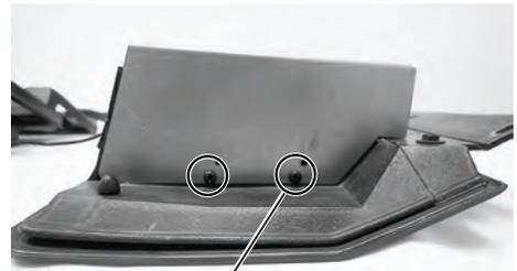
Install glove box cap using (4) #6 x 3/8" pan head screws
