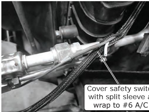
Cover safety switch wire with split sleeve and tie wrap to #6 A/C hose
