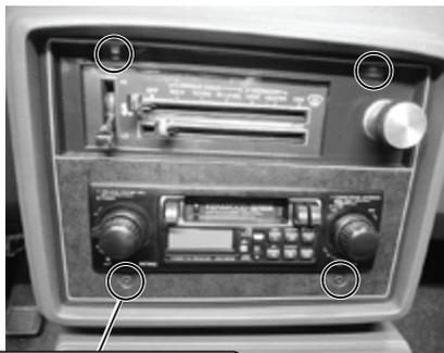
Remove control panel/radio bezel by removing (4) screws
