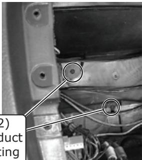
Remove (2) evaporator/duct work mounting screws
