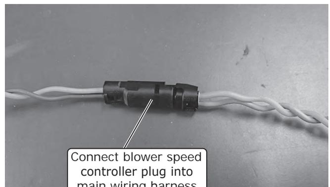
Connect blower speed controller plug into main wiring harness plug
