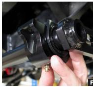
6. Next, it is time to mark the frame, but first, make sure the car is sitting at ride height. Slide one billet sway bar mount over the bushing then raise the bar up to the frame and make a mark for the two holes. Do the same for the other side. (Photo F) and (Photo G)
