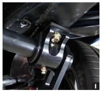
8. Once all four holes have been drilled, use the supplied bolts, nuts, and washers to mount the sway bar to the frame. (Photo I)
