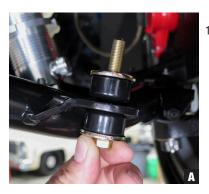
1. Begin by installing the sway bar end link on each side as shown. The end link mounts to the control arm in the factory location using a bolt with two bushings and two washers. (Photo A)
