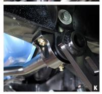
The installation is complete once you have tightened all hardware and greased the sway bar mounts using the supplied grease fittings. (Photo K)
