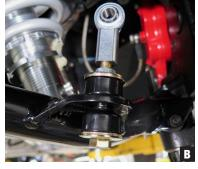
Attach the sway bar to the rod end on both sides using the supplied hardware. Having a second set of hands will make this process much easier. (Photo C)
