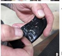
Before installing the sway bar bushings, notice the grooves inside the D-Spec bushings. This design is to help retain grease for extended service life. (Photo D)
