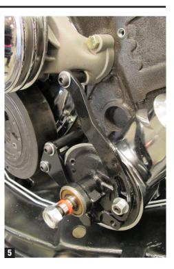
Verify the fit of your belts with the bracket positions; tighten all bolts/nuts and adjust the belt tension as normal.
