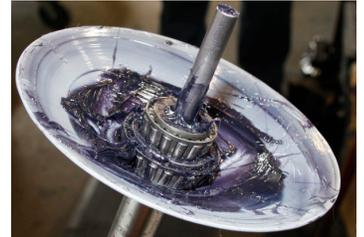
5. Install the aluminum hub onto the spindle. Install the outer bearing, spindle washer and spindle nut. Adjust the wheel bearings as follows:
