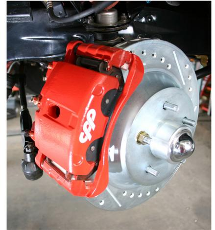
7. Remove the rear steering arm bolt to allow the steering arm to drop down. Install the caliper onto the caliper bracket and tighten down the two caliper bolts.
