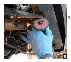
The most effective method we've found for removing old rivets is to cut them down the center with a cutoff wheel (Photo E), remove the rivet head with an air hammer (Photo F) then drill out the remains.
