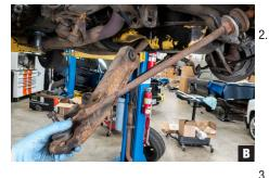
Then remove the front strut rod nut followed by the lower control arm bolt and remove the assembly as one piece (Photo B).
