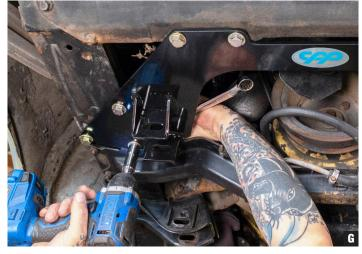
7. Install the Mini Sub-Frame plate using the supplied hardware in the 10 holes left from the rivets (Photo G).
