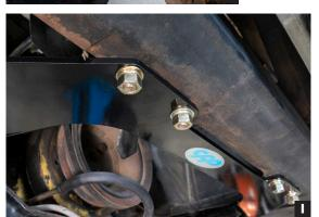
9. If more room is needed to keep the radiator from touching the Mini Sub-Frame hardware, simply remove the front four bolts and nuts then re-install with the nuts on the bottom side of the crossmember as shown (Photo I).
