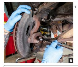
Begin by removing the lower ball joints from the spindle (Photo A). Loosen the castle nut on the ball joint stud but leave it installed a few turns. A handful of whacks with a large hammer usually does the trick to break the ball joint stud loose from the spindle.
