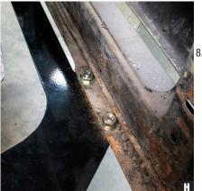
Test fit your radiator, checking for clearance against the front four bolts (Photo H).
