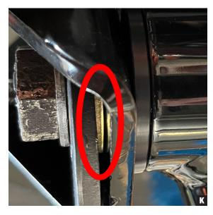
12. Make sure to use a washer between the cam washer and the mounting surface on each of the four sides (Photo K).
