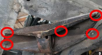
5. Prepare to remove the factory strut rod mounts on both sides. Each mount is held in place with five rivets (Photo D).
