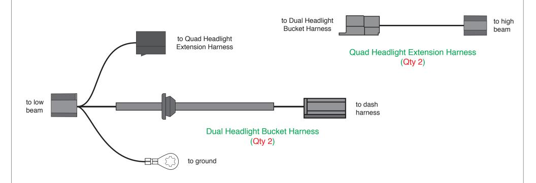
1. There are 2 dual headlight bucket harnesses (used on all vehicles) and 2 quad headlight extension harnesses (used on the 1958-60 vehicles) included in this kit.
