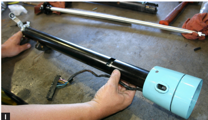
CPP column shown assembled with the factory shift collar and turn signal housing. (FIG. I)
