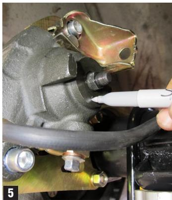
4. Using a 9/16 wrench with the nut reinstalled, adjust the shaft in and out (moving the shaft opposite the direction it travels during operation) until you can clock the lever snug against the caliper
