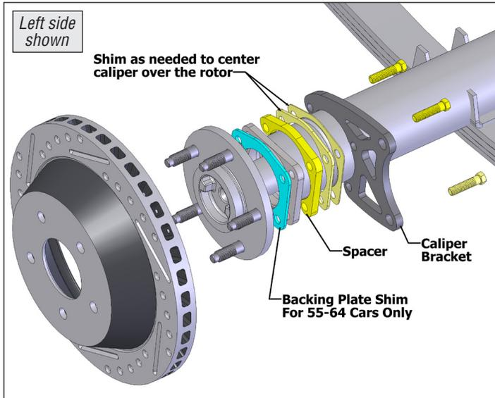
**Note:** Due to variations in the caliper castings, you may need to file down a small amount of metal on the bridge of the caliper if it rubs the outer edge of the rotor. See picture at right.
