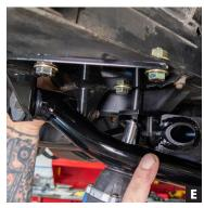
Use a wrench to hold the Nylock nuts while tightening the bolts from the bottom (Photo E).
