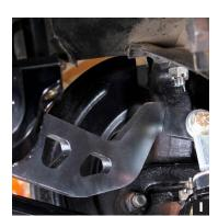
9. Installation Note: The stiffness of the sway bar can be adjusted by switching the installed location of the end link on the laser-cut arms. Installing the end link using the hole closest to the sway bar tube will result in a slightly stiffer ride while the hole further from the tube will yield a softer ride (Photo I).
