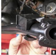
Begin by installing one bushing near the end of the sway bar tube in preparation for mounting the bar to the chassis (Photo B).
