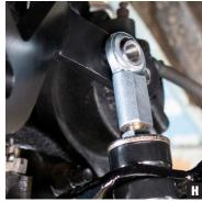
Next, install the rod end but leave it loose until both end links have been installed (Photo H).
