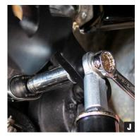
10. Using the supplied hardware, attach the rod end to the laser-cut sway bar arm in one of the two holes (Photo J).
