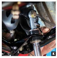
11.Once both end links have been installed, proceed to tighten the jam nuts; then tighten the rod ends (Photo K).
