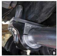
4. Hold the bar up into place against the chassis crossmember and mount the bar utilizing the existing holes (Photo D). Use the supplied Nylock nuts to secure the sway bar mount.
