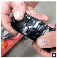
Before beginning the install, note the inside of the supplied sway bar mount bushings. The pockets in the bushings are designed to retain grease for extended service life (Photo A).
