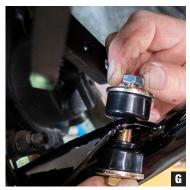
Begin assembling the end links with a bolt, washer, and bushing on the bottom of the control arm; then a bushing, washer and jam nut on top (Photo G).
