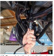
12.Complete the installation by greasing the two sway bar mount bushings (Photo L).
