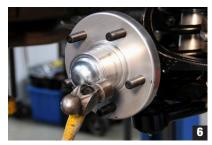
Install the dust cap by tapping around the edge of the cap using a small hammer until fully seated. (Photo 6)
