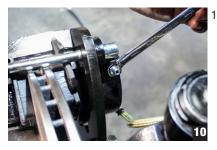
Install the provided bleed screw into the top hole of the caliper and do not overtighten. (Photo 10)
