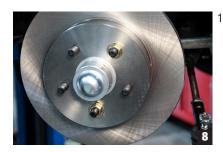
Slide the new rotor onto the hub and use two wheel nuts to hold it in place until the caliper is installed. (Photo 8)
