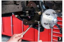
Install the caliper mounting bracket on the inside of the spindle as shown. Torque bolts to spec. (Photo 7)
