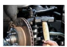
TECH TIP: If the orientation of the hole in the ball joint stud is undesired, vou may remove the castle nut and break loose the ball joint stud from the spindle. Then,
