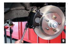
Install caliper to the mounting bracket and torque to spec. Make sure the rotor spins freely. (Photo 9)
