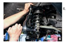
Install the new spindle on the lower control arm first, then the upper control arm. Reuse the old castle nuts and torque to spec. Make sure to use new cotter pins. (Photo 4)
