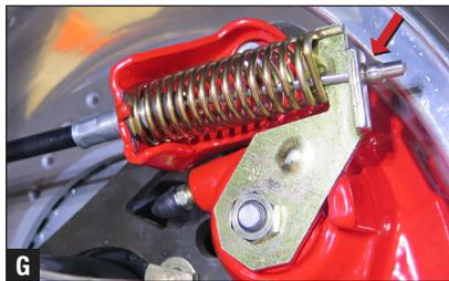
13. Connect the front brake cable pull to the new parking brake cables using the required method for your application. Adjust cable tension as necessary and evenly throughout the cable system so there is no slack. Make sure that the brakes are not applied when the emergency brake is released.
