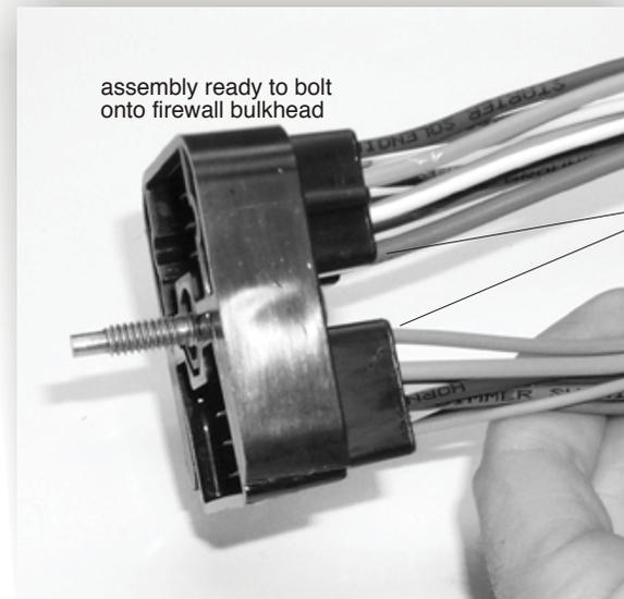
The bulkhead connector from this front light kit must snap into the mating front light connector (bag L), as shown. After snapping together, then bolt the assembly into the dash harness firewall connector using the attached bolt.
