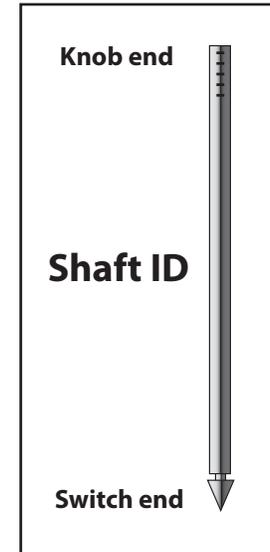
3. Remove the shaft and trim at mark. The shaft can be released from the switch by pulling it outward (toward the rear of the vehicle). Once fully in the "On" position, press and hold the release button on the base of the switch body. Once button is pressed, continue to pull the shaft outward. New switches may be tight, and it might be necessary to move the shaft side to side slightly while pulling to release.
