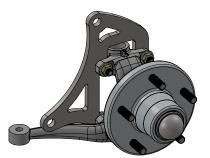
7. Place the rotor over the hub assembly.
