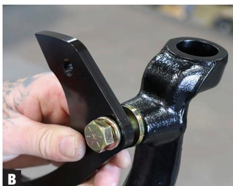
3. Install the caliper bracket to the top of the spindle with the 3/16" spacer and lock washer as shown and leave hardware loose (Photo B).
