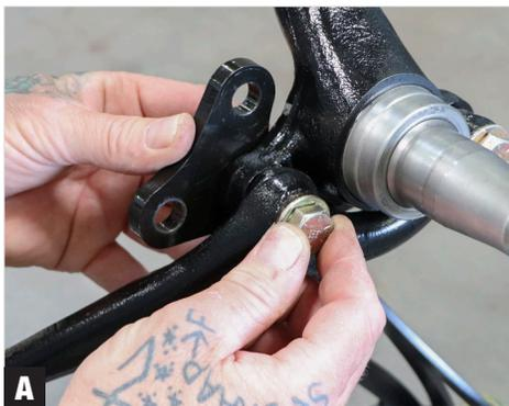
2. Unbolt the steering arm and then attach the three-hole spindle bracket using the supplied hardware but do not fully tighten (Photo A).
