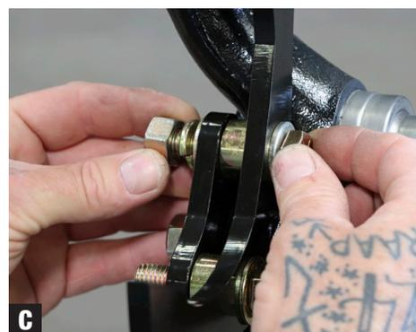
4. Bolt together the spindle bracket and caliper bracket with the two 1/2" spacers in between (Photo C).
