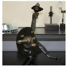
the rear of the car. The bracket mounts on the same surface the original backing plate was mounted on to. Refer to images as needed.
