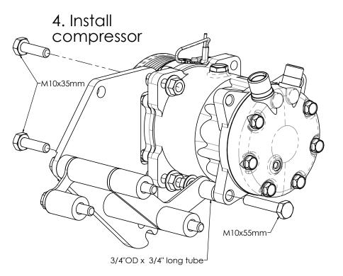
Tighten 10mm fasteners to 37 ft-lbs (50 N-m)
