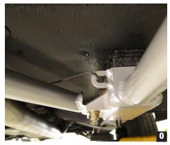
13. Re-attach the parking brake return spring using the integrated tab on the Subframe connector. (Fig 0)
