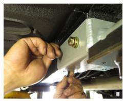
Tighten down exterior sides and repeat steps for the inside-facing mounting holes. (Fig I)
