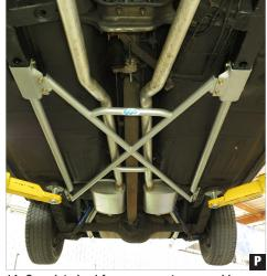
14. Completed subframe connector assembly shown with optional CPP X-Frame Brace #6570XFB-S. (Fig P)
