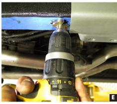
Mark and drill a 7/8" hole, 3/4" forward of the subframe connector's mounting bracket—this will provide access into the rail to allow the mounting hardware backing plates to be inserted. (Fig E)
