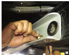
11. Drill the two 3/8" holes for the mounting hardware and install backing plates. (Figs L-M)
