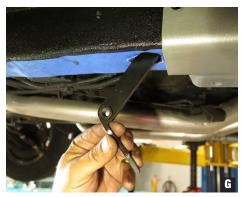
7. Insert the backing plate ("holding" tabs will point in, towards each other) and attach with supplied hardware. (Figs G-H)
