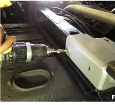
With the bar completely compressed onto the box rail, drill the two outer holes using a 3/8 bit. (Fig F)
