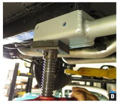
Rotate the bars forward and align onto the sheetmetal box rails; use jack stands to support the bars. On passenger side, undo parking brake return spring, as it will interfere with placement. (Fig D)
