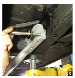
With the slotted holes facing downward, attach the Subframe connector bars to the forward leaf spring mount using the stock hardware on '641/2 - 66 models; use supplied spacers/bolts on '67-70 models. Leave semiloose. (Fig C)
