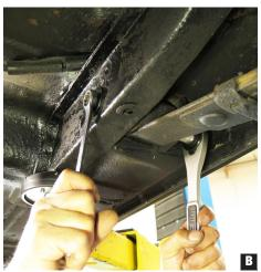
2. As a precaution, take weight off rear end prior to removing the forward leaf spring eyelet bolts, which will initially locate the Subframe connectors in the rear. (Figs A-B)
