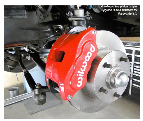
9. Bleed the front brake system with quality brake fluid.
