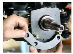
1. Start by removing either the factory drum brake assembly or your current disc brake conversion from
