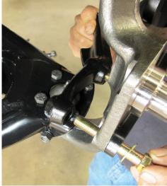
Note: When "stock-offset" hub/rotors are used, the bolts must be installed with the nuts **behind** the spindle.
