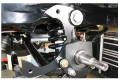
Tighten down the top anchor bolt and bracket bolt now.
