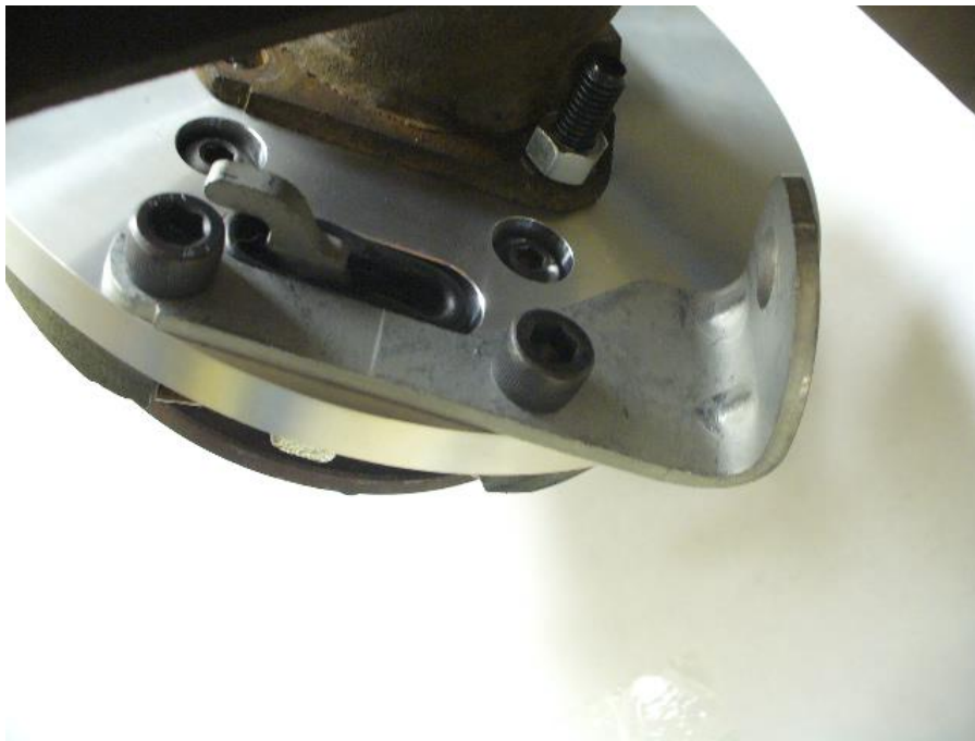
Figure 4: Park assembly installed on driver's side (Actuator is shown at the bottom)
