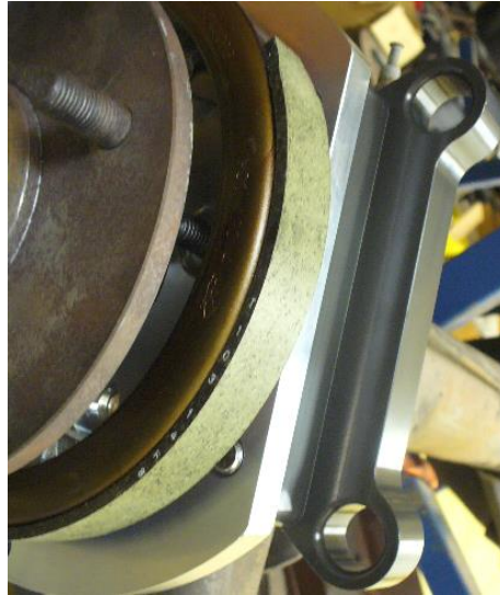
Figure 3: Park brake assembly correctly installed
