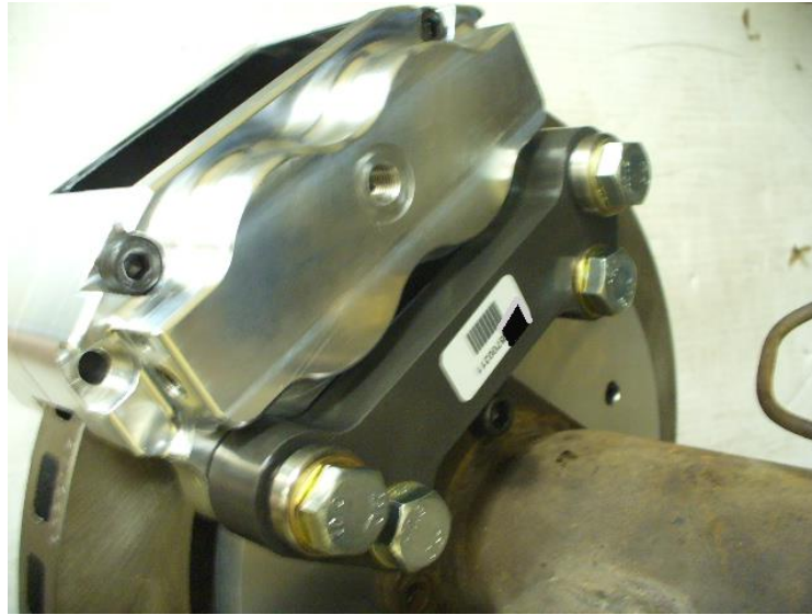
Figure 5: Caliper installed on intermediate bracket
