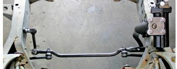
bushing and spring and tighten the end cap screw and install the cotter pin. Install the washer and nut along with the cotter pin on the idler arm. Install the tie rod ends onto the new center link. Once all your toe adjustments are done, tighten the castle nuts and install the cotter pins. Make sure you grease the zerk fittings on the ball joints, idler arm and tie rod ends.
